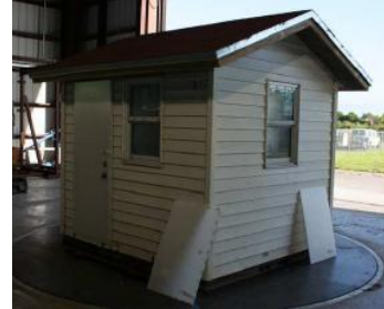
Figure 13: Test house showing installed Storm Stoppers Original 3/8 in. door panel and window panels before installation (Right Side)
