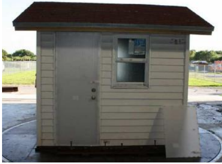
Figure 11: Test house showing installed Storm Stoppers Original 3/8 in. door panel and window panel before installation.
