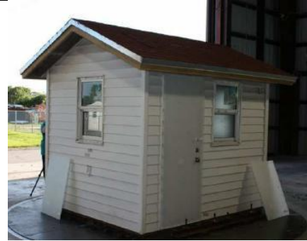
Figure 12: Test house showing installed Storm Stoppers Original 3/8 in. door panel and window panels before installation (Left Side)
